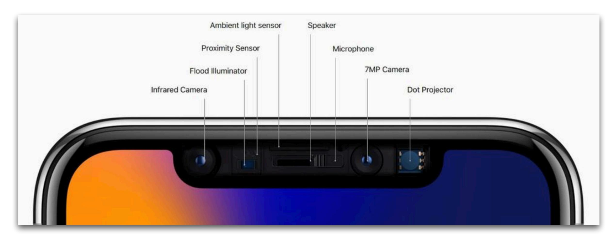
Apple shrunk the Kinect, plus a **lot** more, into the Face ID module of iPhone X measuring 5mm x 25mm
